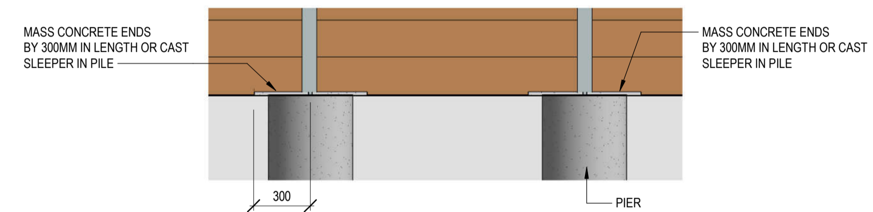
5 BASE FIXING DETAIL (A1) 1:20
