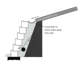
Link Blocks: Link blocks come in a variety of shapes and sizes. A traditional diamond style link block tapers back layer by layer. Most councils will require certification for walls built over 1m in height. Link walls such as the Windsor Block from Adbri Masonry are engineered to be built up to 1 m in height.
