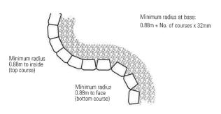
All cores and voids between units to be filled with infill
